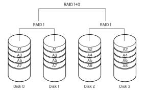
If a drive failure occurs, subsequent read and write operations are directed to the other surviving drives. A replacement drive can then be rebuilt using the data from the surviving drives. Also, because data is duplicated on the primary and additional drives, four 120 GB collectively have a maximum of 240 GB on which to store data.
